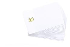
The SLE4428 is a standard, low-cost EEPROM memory smartcard with 1K bytes of available storage, an irreversible write protection feature and a 2-byte programmable security code.
